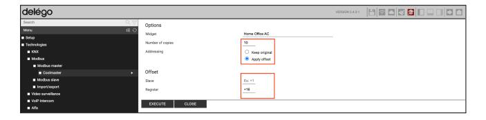
When done, return to the Modbus line page, and change the names of the AC units in the WIDGETS list. Finally, press STOP and START buttons to restart the communication; if everything has been correctly set, the "dots" in the detail page of each AC unit must pass from red to green color.
