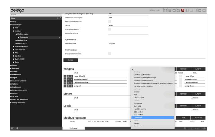
and press the ADD button; a new widget will be added to the list above, for the first AC unit. Access its detail page, enter a name and "1" as address, by leaving all the other settings as default:
