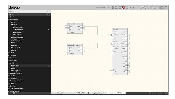
Delégo automatically converts KNX into Modbus commands, and vice versa.
