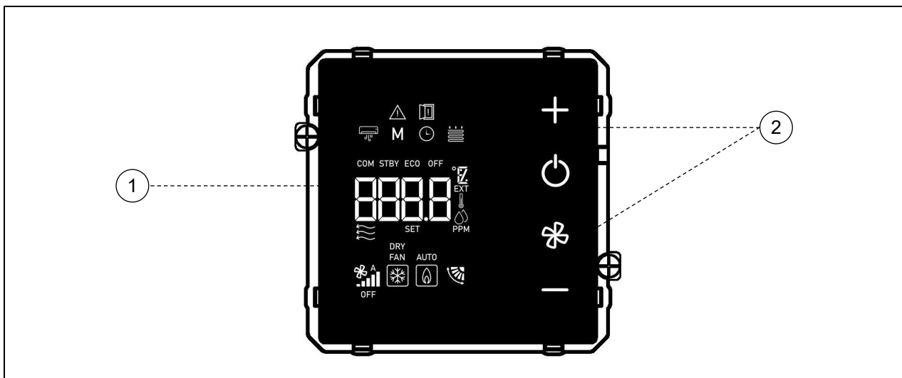
Figure 4 - User interface: display (1) and backlit touch LEDs (2)
