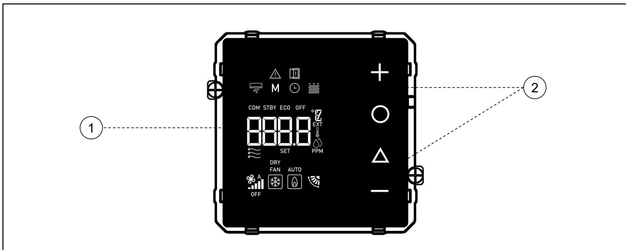
Figure 4b - User interface Classic version: display (1) and backlit touch LEDs (2)
